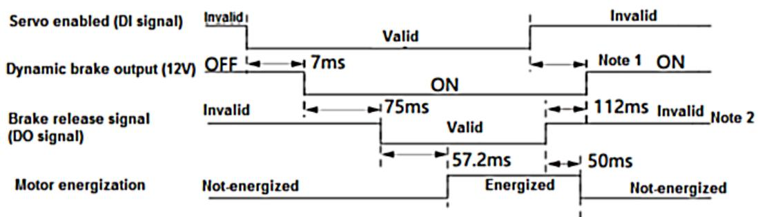
Note 1) When motor stops, the time sequence of dynamic brake output is related to the motor running speed. The greater the speed, the greater the time sequence. And the minimum value is 400us.
