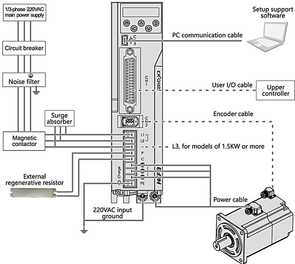
※A twisted-pair shielded cable should be used if I/O cable length is over 50cm.
