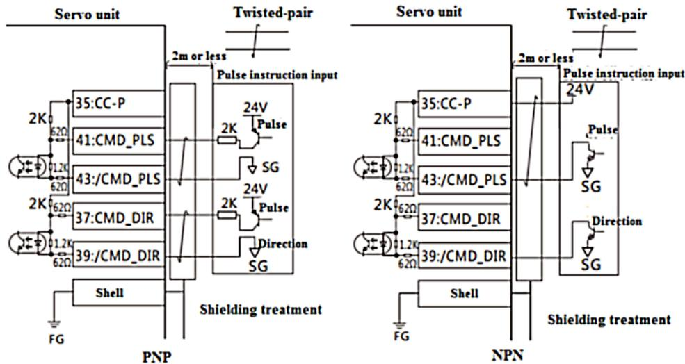
Note 7: If 5V open-collector circuit is required, be sure to connect an external 300Ω resistor.
