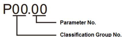
The first row displays parameter group No. and offset, e.g. **P0100**, and the rightmost digit flickers to be modified.
