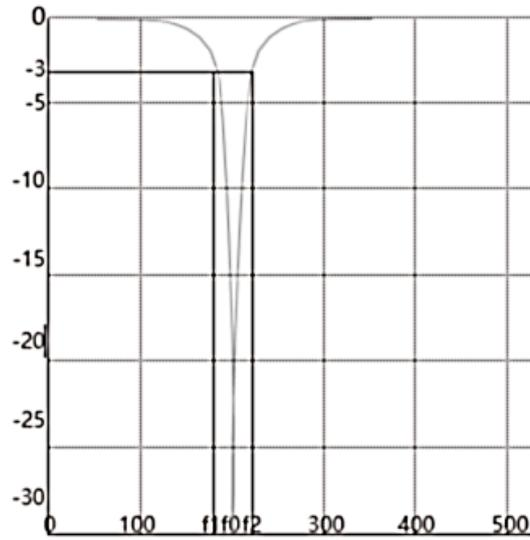
Notch filter frequency is  $f_0$ . Notch filter width  $K_w = (f_2 - f_1) / f_0$ .
