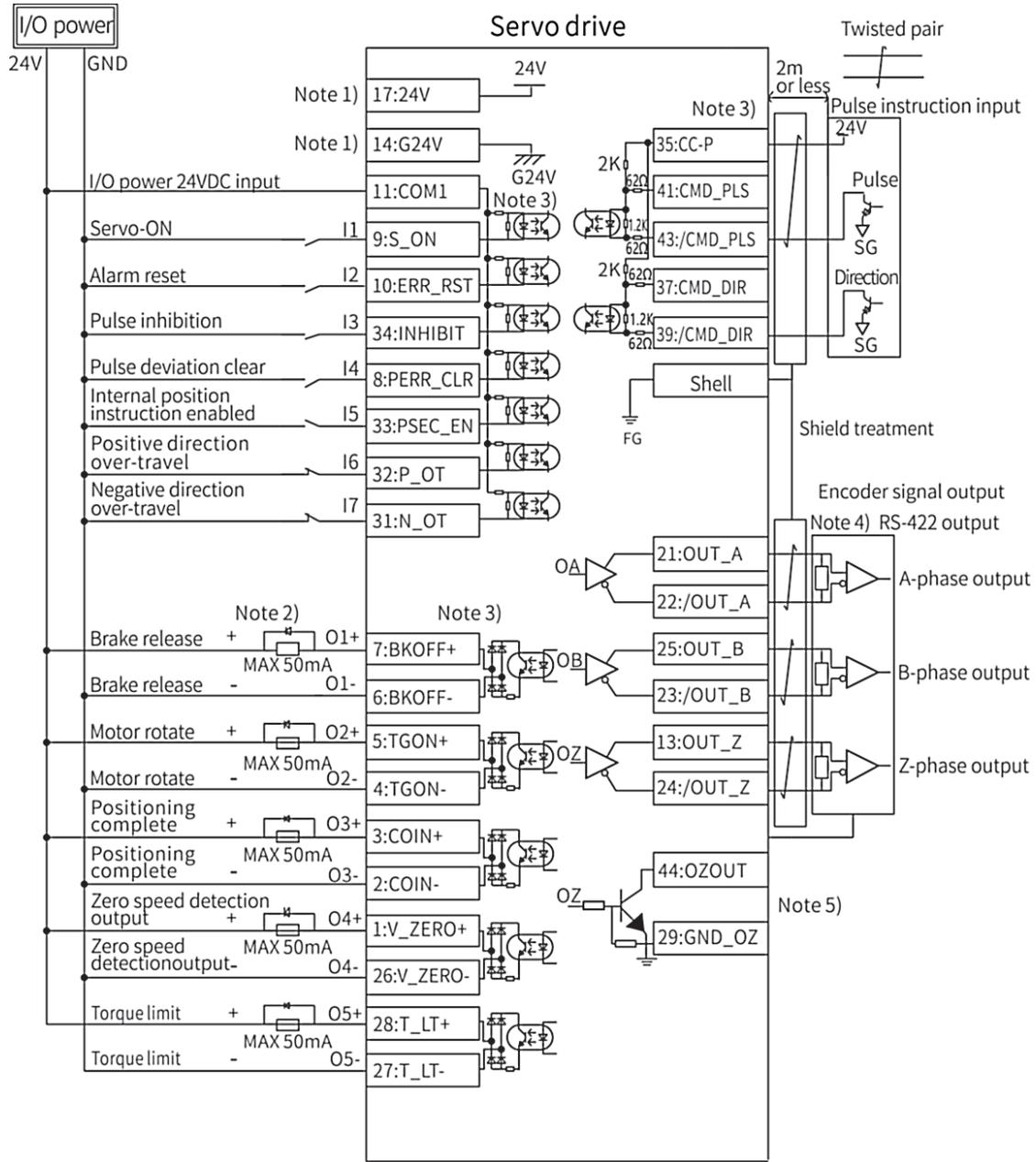
Note 1: Internal 24V power (24V, G24V) can be used as I/O power. But the maximum output current is 150mA, and when driving the output such as relay and brake, please use external independent power.
