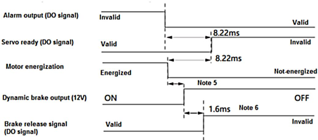
Note 5) When motor stops immediately, the time sequence of dynamic brake output is related to the motor running speed. The greater the speed, the greater the time sequence. And the minimum value is 500us.
