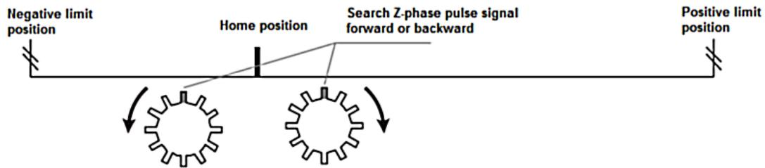
Figure 6-11 Search Z-phase pulse signal forward or backward
