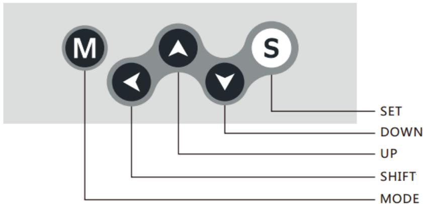
MODE button (m): switch level of parameters.
