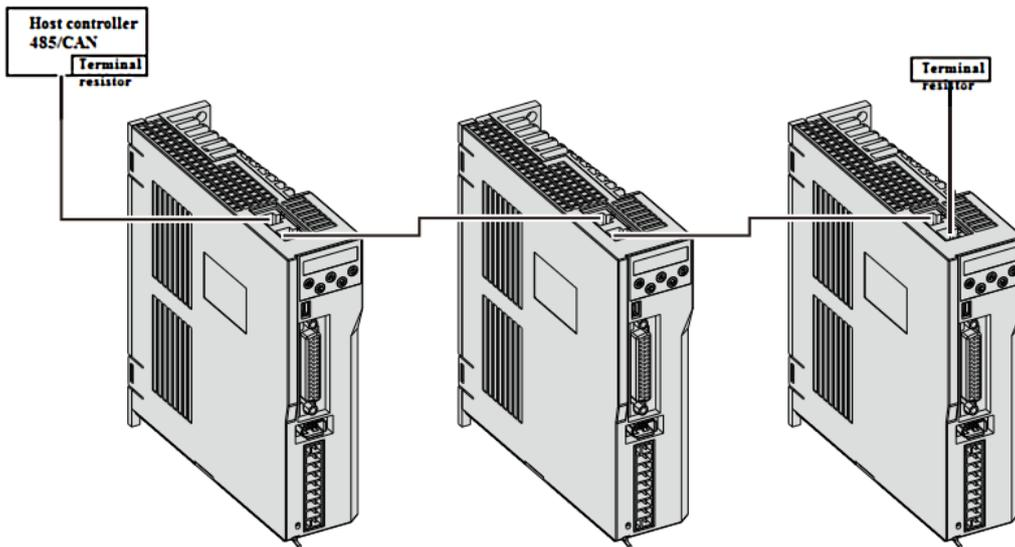
L1=5m (max): cables between upper controller and servo drive should be less than 5m.
