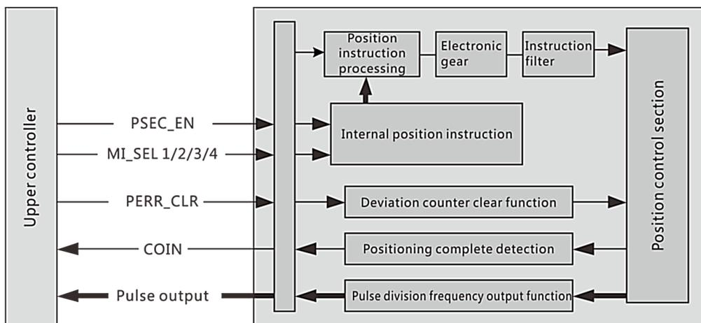
Figure 6-4 Block diagram of internal position control
