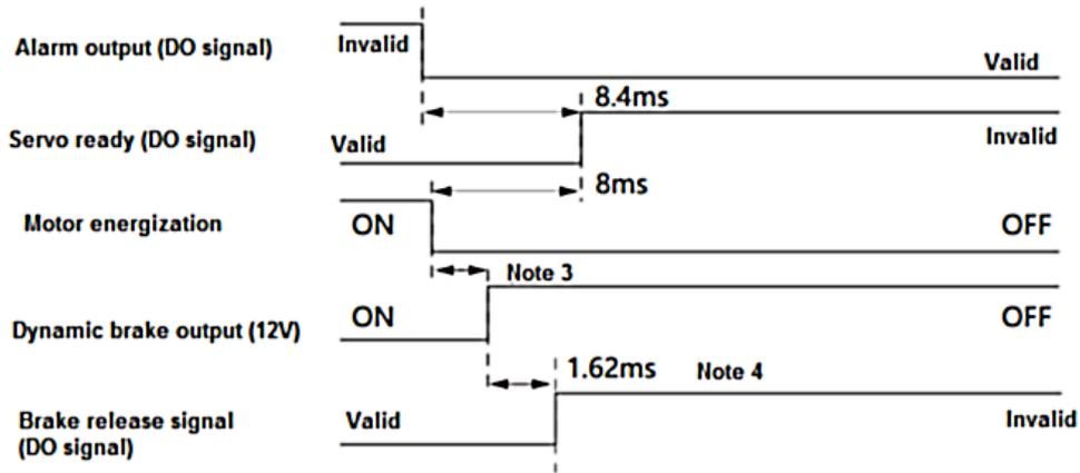
Note 3) When motor stops, the time sequence of dynamic brake output is related to the motor running speed. The greater the speed, the greater the time sequence. And the minimum value is 500us.
