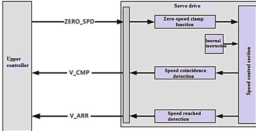
Figure 6.2 Block diagram of speed control mode
