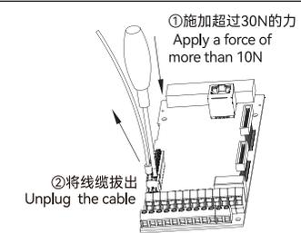
4.6 主回路接口 线缆拆装 4 (Main circuit interface, cable connecting and disconnecting 4)
